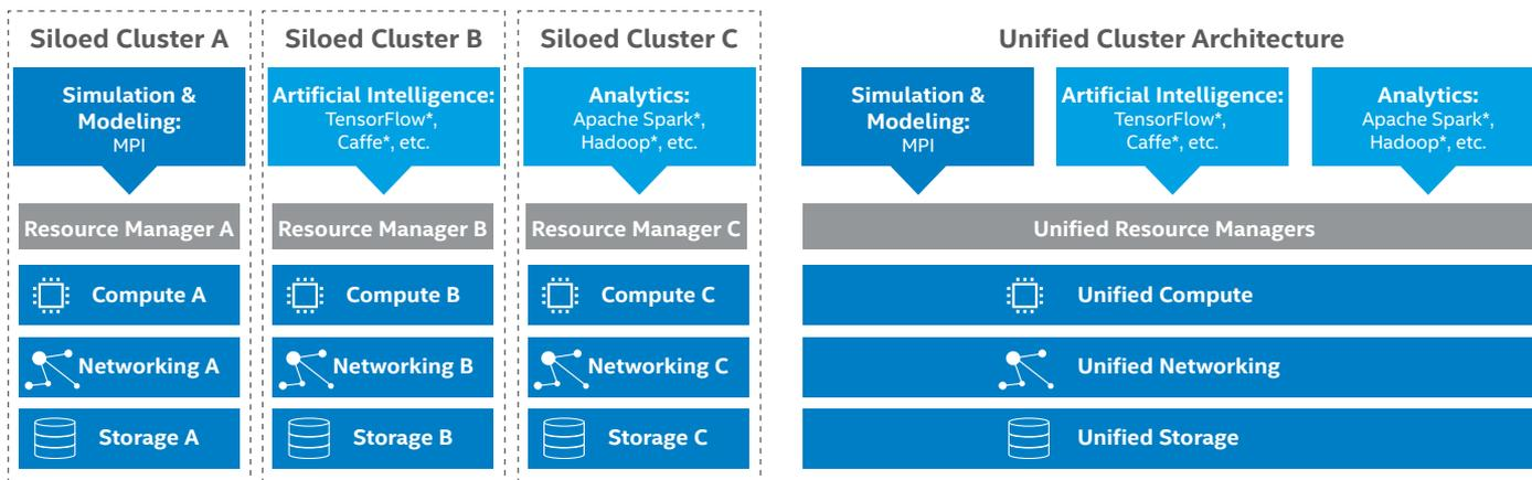
Figure 1. Siloed versus unified cluster architecture for simulation and modeling, AI, and analytics workloads.
