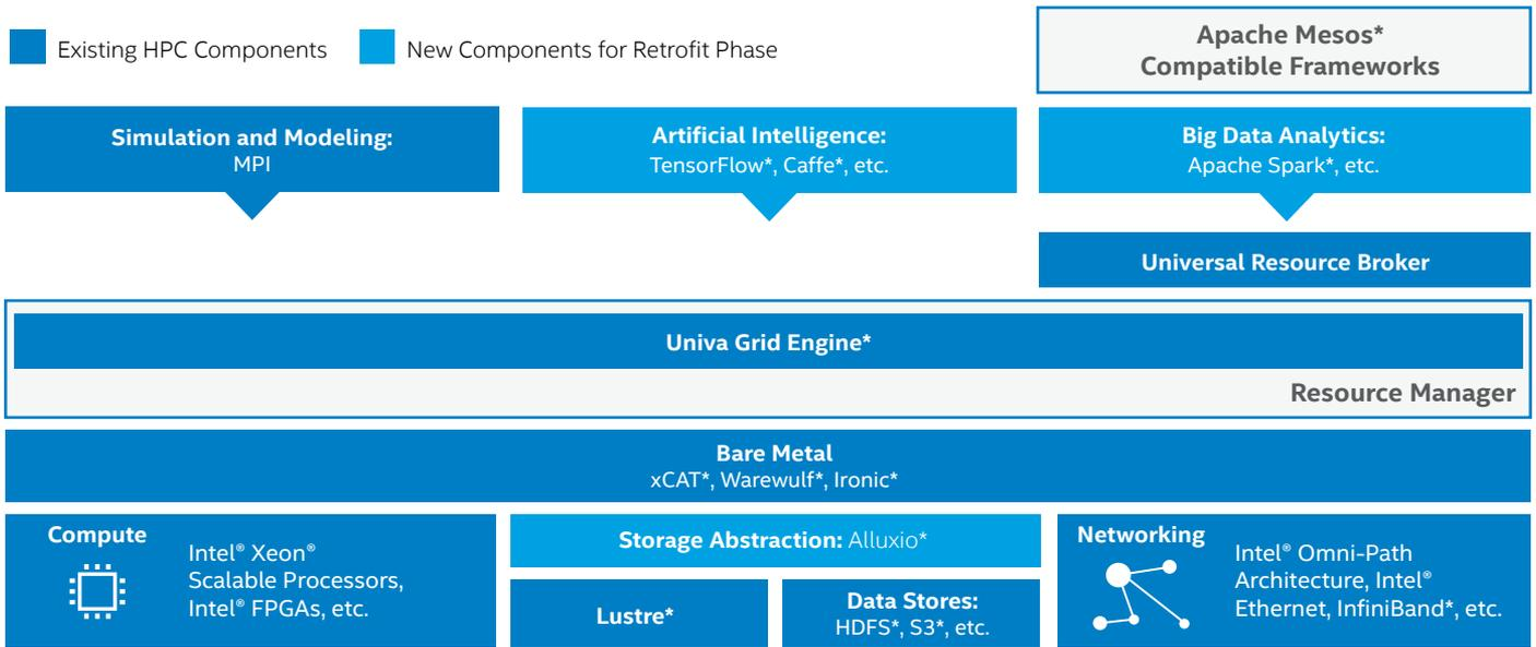
Figure 3. Solution 2: Univa\* Grid Engine and Resource Broker.
