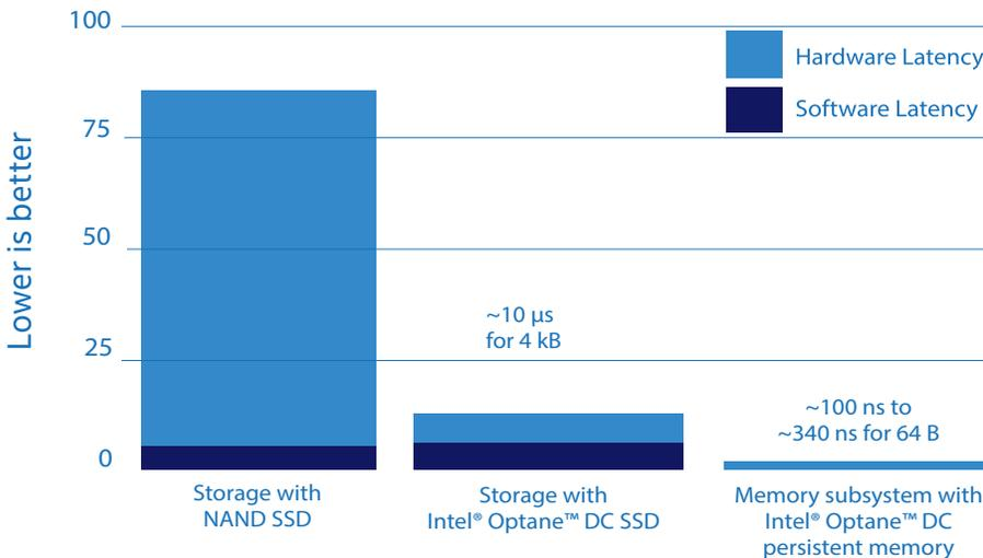
Figure 3. Comparison of read latency for NAND SSDs, Intel® Optane™ DC SSDs, and Intel Optane DC persistent memory.<sup>2,3</sup>
