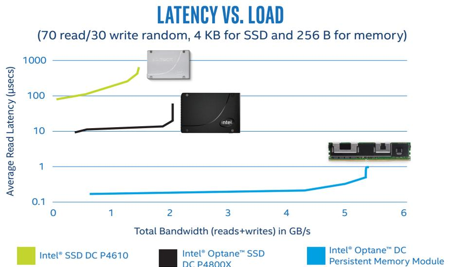
**Figure 5.** Comparison of the loaded latency for Intel® NAND SSDs, Intel® Optane™ DC SSDs, and Intel Optane DC persistent memory.<sup>1,3</sup>
