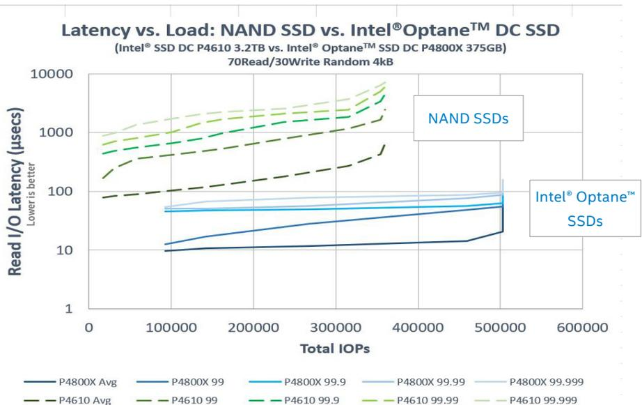
**Figure 1. Intel Optane SSDs deliver much lower latency at load than NAND-based SSDs<sup>1</sup>**
