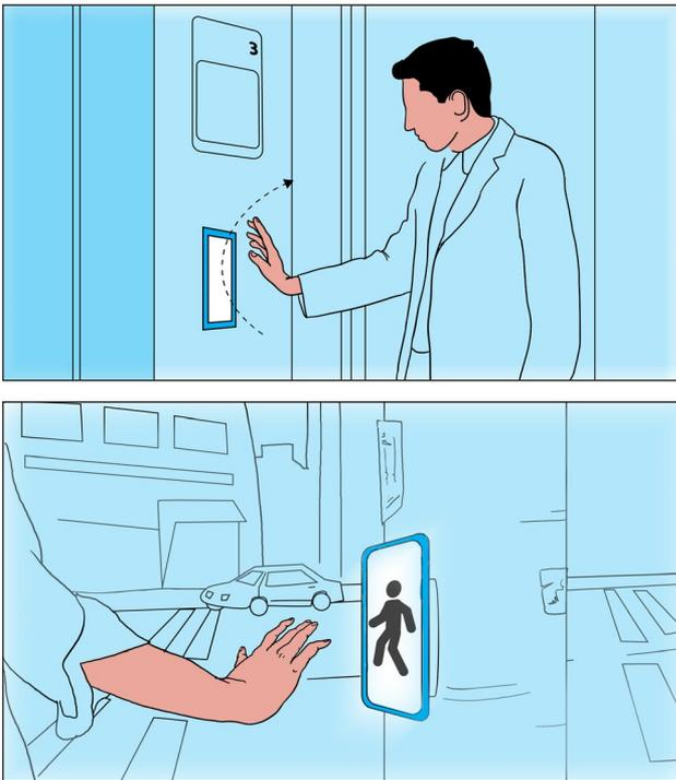
Figure 1. Millimeter wave radio as presence detector
