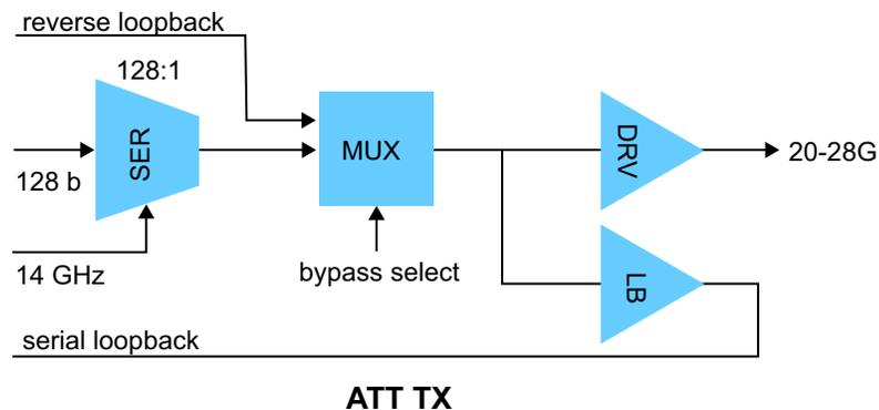
The clocking scheme for the 28 Gbps serializer uses a similar architecture as the one used in the 14.1 Gbps channel for 28 nm Stratix V FPGAs. A shared LC PLL is used in Stratix V FPGAs to generate a raw 14 GHz clock.
