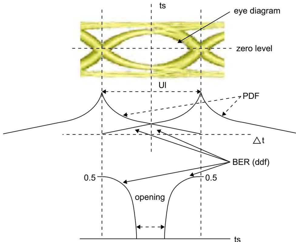
The BER of the overall link system depends on the jitter, noise, and signaling performances of its subsystems, such as the transmitter, channel, and receiver. Altera's innovative design enables the transceiver to meet and even exceed the requirements posed by various high-speed I/O standards. Due to the excess margins in jitter and noise, it also enables users to design systems with lower costs and better BER system performance.
