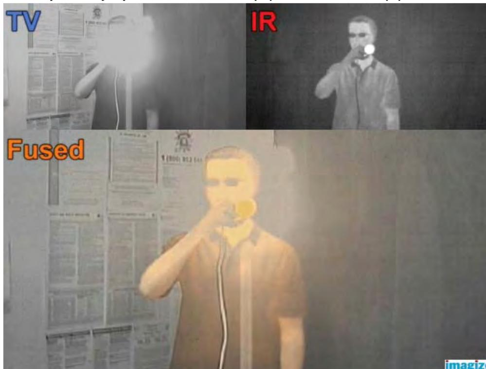
While the visible image (Figure 8, top left) contains information about the surroundings, the thermal image (Figure 8, top right) only shows discernible features where the temperature differs from the background. Conversely, the performance of the thermal sensor is unaffected by the strong light source, while the visible sensor provides no information in the same area due to saturation.
