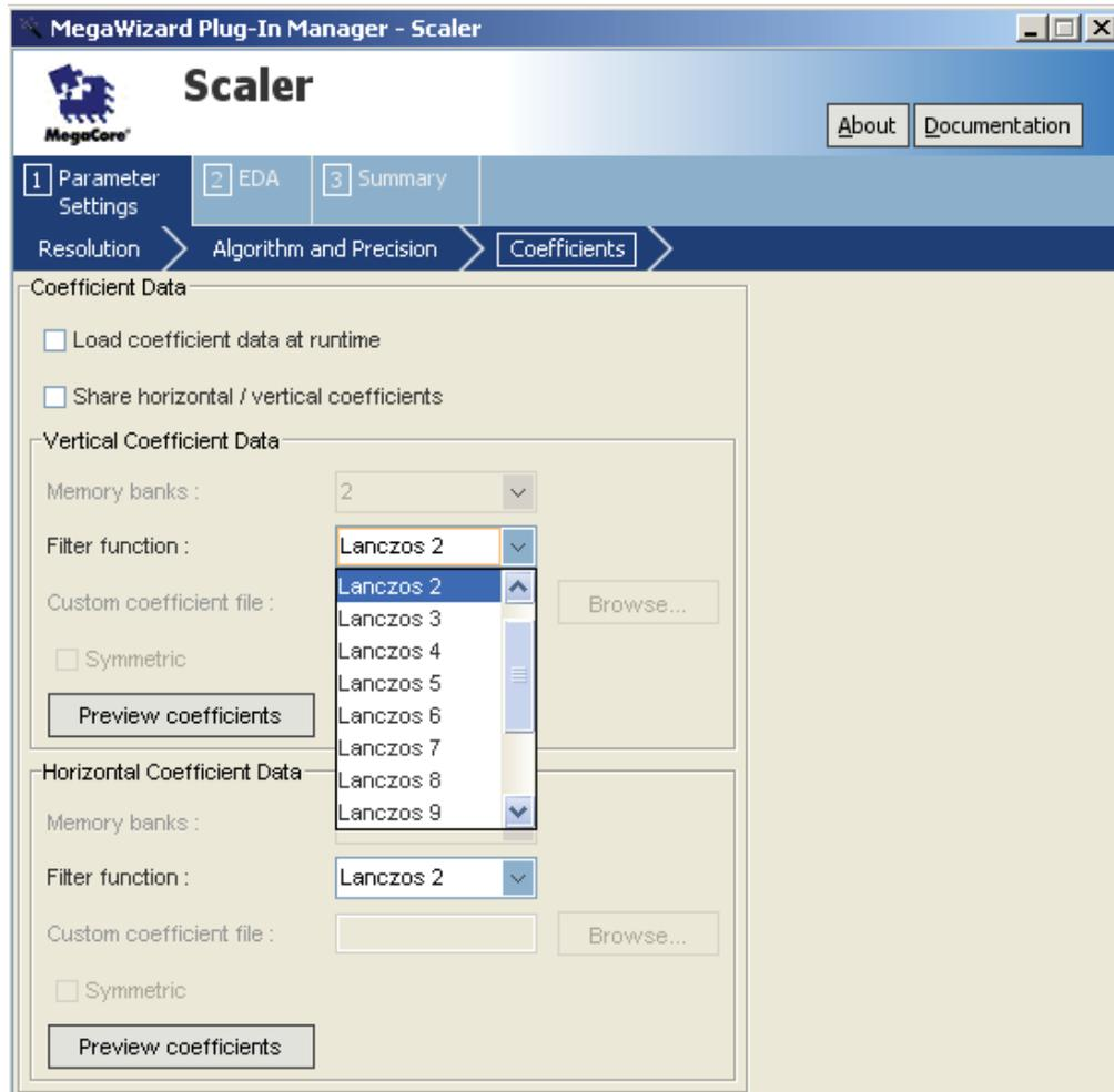
A designer can either select from a range of Lanczos algorithms to scale the image or bypass these altogether in favor of custom coefficients. In either case, the function automates the tedious job of generating the HDL code for what is essentially a two-dimensional filter. It then maps it to FPGA structures such as the digital signal processing (DSP) blocks and the embedded memory blocks, thus improving productivity and reducing design time.
