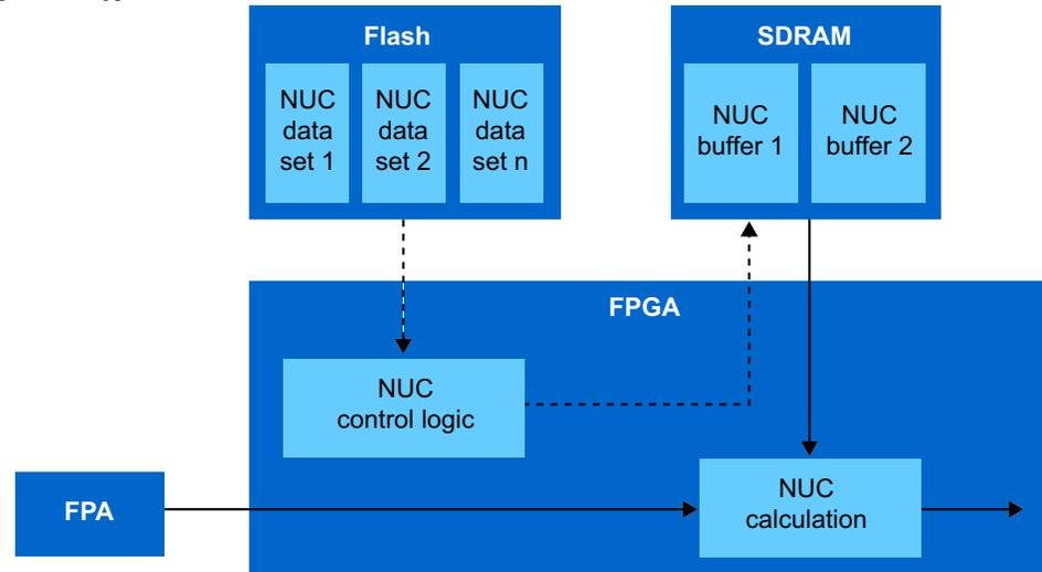
This relatively simple example shows how the flexibility of the FPGA routing fabric provides highly efficient ways to move data without creating architectural bottlenecks. This flexibility allows the designer to create data pathways that fit the algorithm rather than change the algorithm to fit a pre-defined architecture. Flexibility is a key advantage of FPGA solutions compared to processor-based systems and is critical for achieving very low power consumption.
