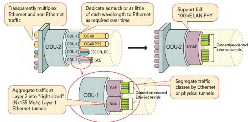
FPGAs play a vital role in the implementation of this flexible client adoption system across specific optical bandwidth channels. From the OTN implementation point of view, it is a data aggregation of various independent ports to provide the required bandwidth. Table 1 shows the data rates supported by current OTN standards. OTU4 will add a line rate of 100G.
