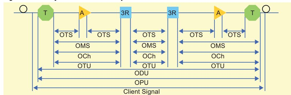
A distinguishing characteristic of the OTN is its provision of transport for any digital signal, independent of client-specific aspects (i.e., client independence). To do so according to the general functional modeling described in Recommendation G.805, the OTN boundary is placed across the optical channel/client adaptation to include the server specific processes and leave out the client specific processes, as shown in [Figure 3](#).
