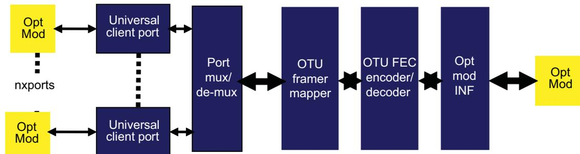
The Stratix IV GX family supports up to 32 transceivers with clock data recovery (CDR) and data rates from 600 Mbps to 8.5 Gbps, plus up to an additional 16 transceivers with CDR, supporting data rates from 600 Mbps to 6.5 Gbps. Stratix IV GX FPGAs also support up to 530K logic elements (LEs), which can support a full 40G muxponder application. [Table 4](#) shows Stratix IV GX transceiver support for various OTN data rates.
