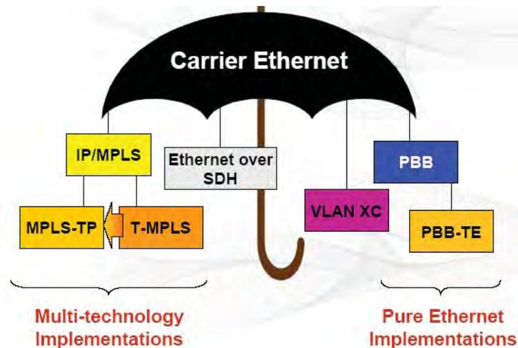
The process of converting Ethernet to Carrier Ethernet Transport started not long ago. So far, the ITU-T has provided options for building an Ethernet service-based carrier network system. ITU-T recommendations deal with Ethernet over Transport (EoT), where transport is a traditional carrier technology such as PDH, SDH, or OTN.
