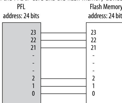
**Figure 8. Micron J3, P30, and P33 Flash Memories in 16-Bit Mode**
