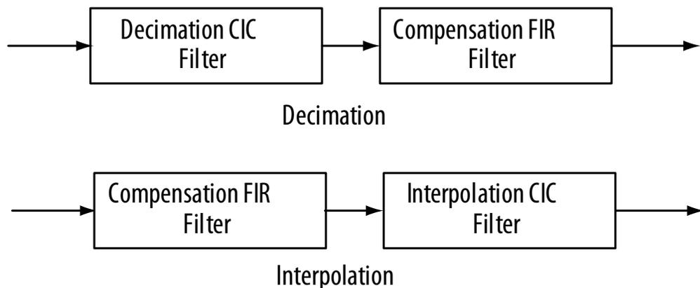
You can use a frequency sampling method to determine the coefficients of a FIR filter that equalizes the undesirable passband droop of the CIC and construct an ideal frequency response.
