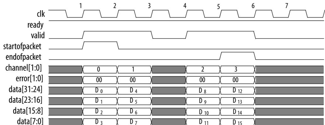
During cycle 1, the CIC IP asserts `startofpacket`, and transfers the first four bytes of packet. During cycle 5, the CIC IP asserts `endofpacket` indicating that this is the end of the packet. The `channel` signal indicates the channel index associated with the data. For example, on cycle 1, the data  $D_0, D_1, D_2,$  and  $D_3$  associated with channel 0 are available.
