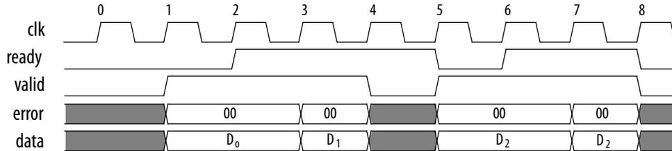
The source provides data and asserts `valid` on cycle 1, even though the sink is not ready. The source waits until cycle 2, when the sink does assert `ready`, before moving onto the next data cycle. In cycle 3, the source drives data on the same cycle and because the sink is ready to receive it, the transfer occurs immediately. In cycle 4, the sink asserts `ready`, but the source does not drive valid data.
