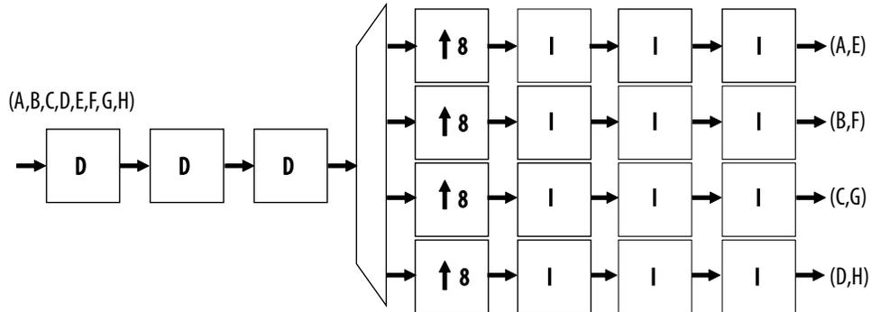
The required sampling frequency of the output data only allows time multiplexes of two channels per bus. Therefore, you must configure the CIC filter with four output interfaces. The rate change factor must also be at least four to exploit this architecture, but this example shows a rate change of eight.
