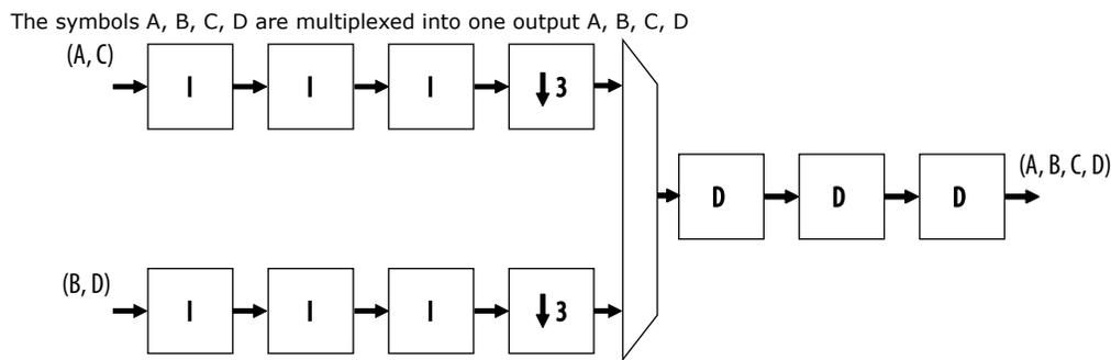
The sampling frequency of the input data only allows time multiplexes of two channels per bus. Therefore, you must configure the CIC filter with two input interfaces. For two interfaces, the rate change factor must also be at least two to exploit this architecture. The CIC support up to 1,024 channels by using multiple input interfaces in this way.
