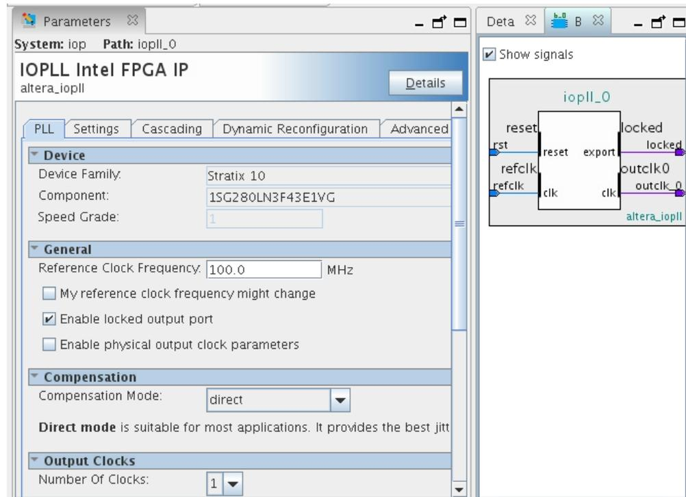
4. Set the parameter values in the parameter editor and view the block diagram for the component. The **Parameterization Messages** tab at the bottom displays any errors in IP parameters:
