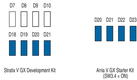
Figure 8. Condition of LEDs for Parallel Loopback Demonstration
