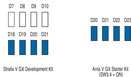
Figure 6. Condition of LEDs for Receiver Demonstration
