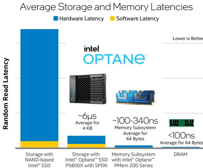
**Figure 4.** Because it resides on the memory bus, Intel® Optane™ persistent memory (PMem) latency is much closer to that of DRAM than to block storage latency.<sup>5</sup>
