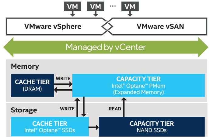
Figure 3. In a tiered memory system, Intel® Optane™ persistent memory (PMem) serves as the main system memory, while the system's DRAM serves as a memory cache.
