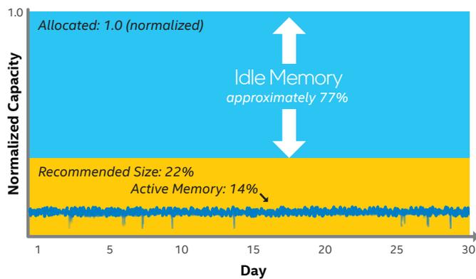
**Figure 6.** The cluster's cumulative VM memory utilization profile shows active data use is well below the allocated DRAM capacity.
