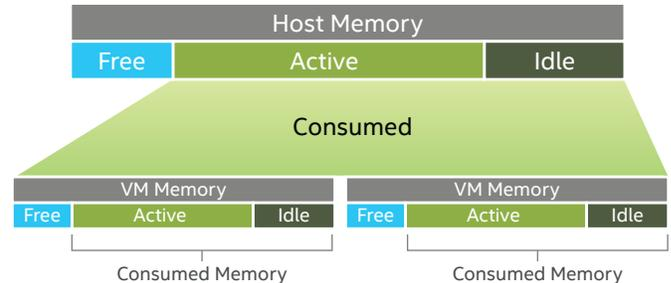
**Figure 5.** Active and idle memory make up a VM's consumed memory, which together with free memory, comprise the total allocated memory for that VM.
