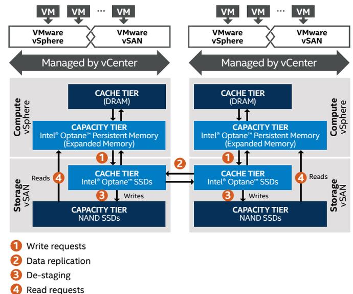
Figure 1. Hardware architecture components and I/O flow.
