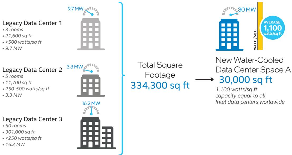
**Figure 1.** When construction is complete, the close-coupled evaporative cooling solution data center will exceed the combined power capacity of all current Intel® data centers. Economies of density work similar to Moore’s Law: the cost per kW goes down as more kW are added to each square foot of production area.
