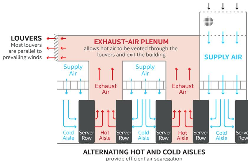
**Figure 6.** Alternating hot aisles (exhaust air) and cold aisles (supply air) provide efficient air segregation, and the exhaust-air plenum allows hot air to easily exit the building. The louvers are positioned parallel to prevailing winds so that the exhaust air can easily exit the building.
